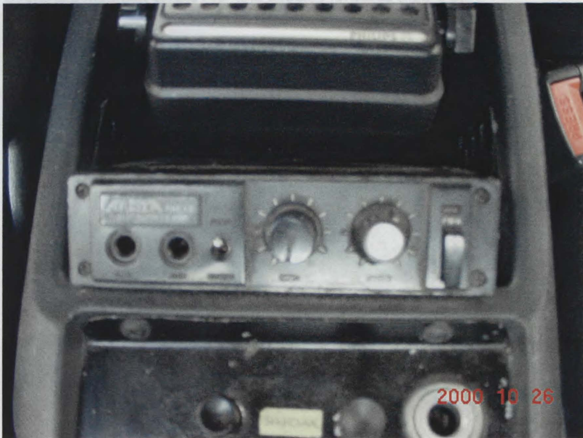
Figure 5 Astra brand electronic sirens control panel
