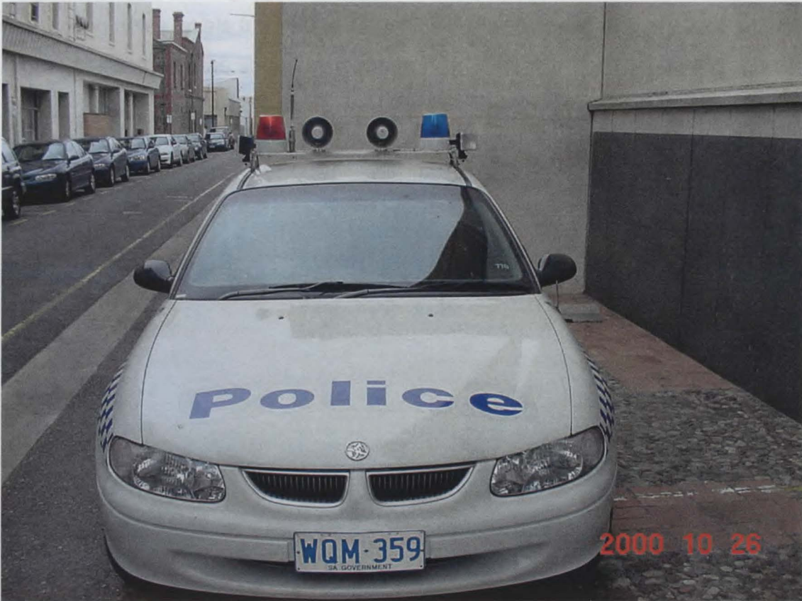
Figure 6. Roof mounted speakers
